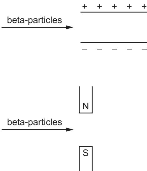
In which direction is the beam deflected in each case?
